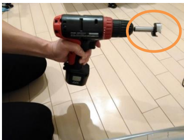
1) Drill with 32-mm Hole Cutter
